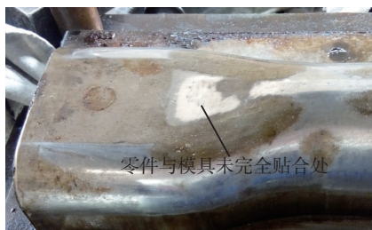
图12 成形模修理 Fig.12 Repair of forming die
