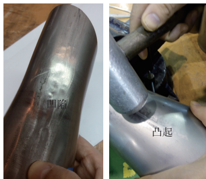
图11 成形后零件的缺陷 Fig.11 Defective parts after forming
