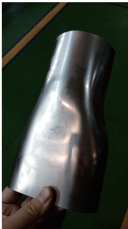
图10 成形后合理的变形 Fig.10 Reasonable deformation after molding
